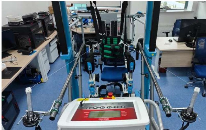
Figure 2: The proposed Robotic Perturbation System (RPS) together with the GEAR Robot
